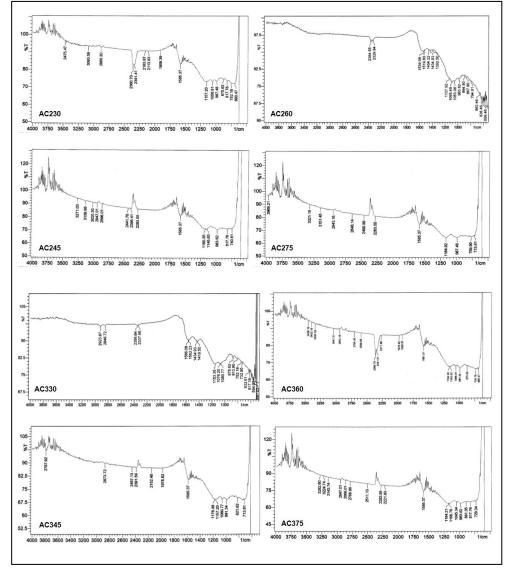
Figure 1. The FTIR spectra for palm kernel shell activated carbons.
